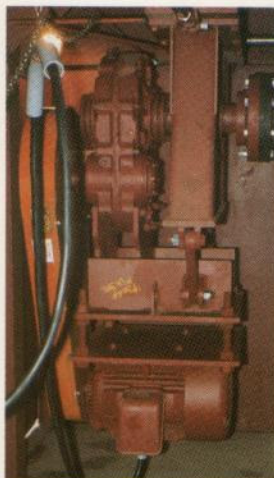
Discharge auger provides a controlled flow of material out one side of enclosure to accumulation conveyor.
