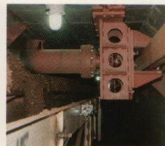
Discharge auger provides a controlled flow of material out one side of enclosure to accumulation conveyor.
